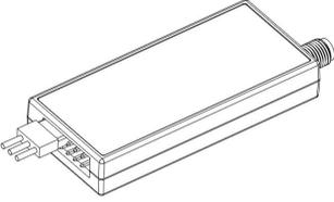
A line drawing of a rectangular R/C receiver with a multi-pin connector on the left side and a single-pin connector on the right side. |
