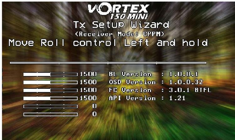
Follow the prompts, ensuring that the correct stick is moved each time. As each control is recognized, it's name will appear to the left of the servo bar.
