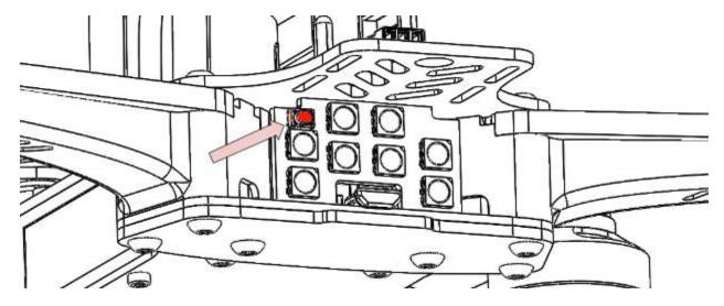
To switch bands, press the button on the LED board for approx. 2 seconds until you hear the first beep, and release.
